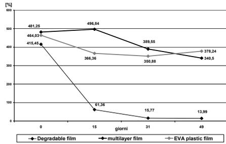
Fig. 9. Extensibility percentage of the films used for solarization.
