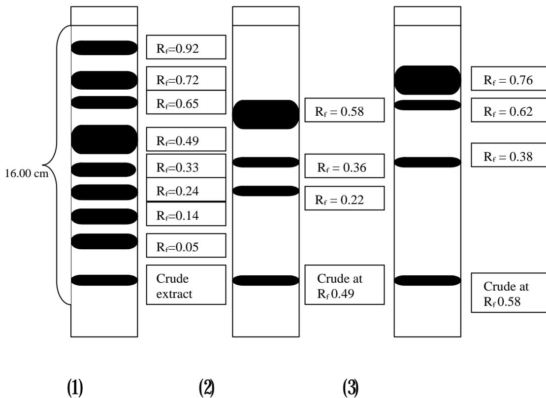
Fig. 1. TLCs of *A. calamus* extract (1), fraction at  $R_f$  0.49 (2) and fraction at  $R_f$  0.58 (3) with UV detection
