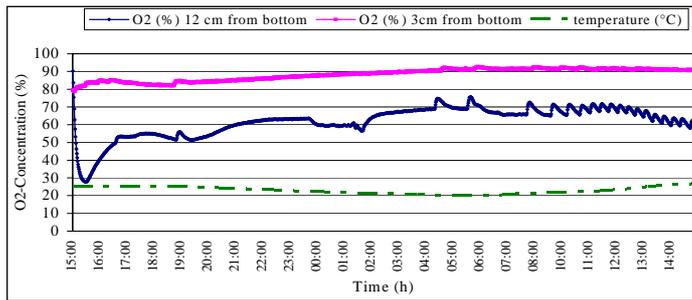
Fig. 4. Daily time course of oxygen concentration and temperature in Perlite filled container.
