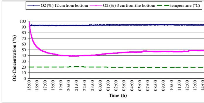
Fig. 3. Daily time course of oxygen concentration and temperature in Coir filled container.
